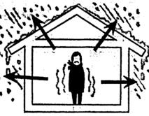
RADIATION: Cold walls create discomfort. They draw heat from the body faster than can be comfortably maintained. The room temperature may be 70 degrees, yet the house feels chilly and drafty.
